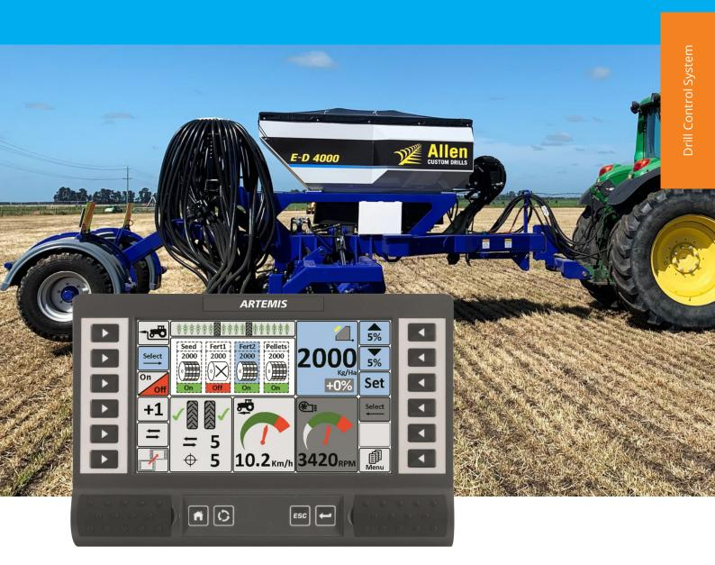
The new generation **RDS ARTEMIS DRILL** control system is a variable rate control and monitoring system for seed drills. The system removes the need for a mechanically driven landwheel by operating the metering unit with an electric motor maintaining its speed proportional to forward speed, or adjusting sowing rates to suit the mapping provided by the precision farming option if this is utilised.
